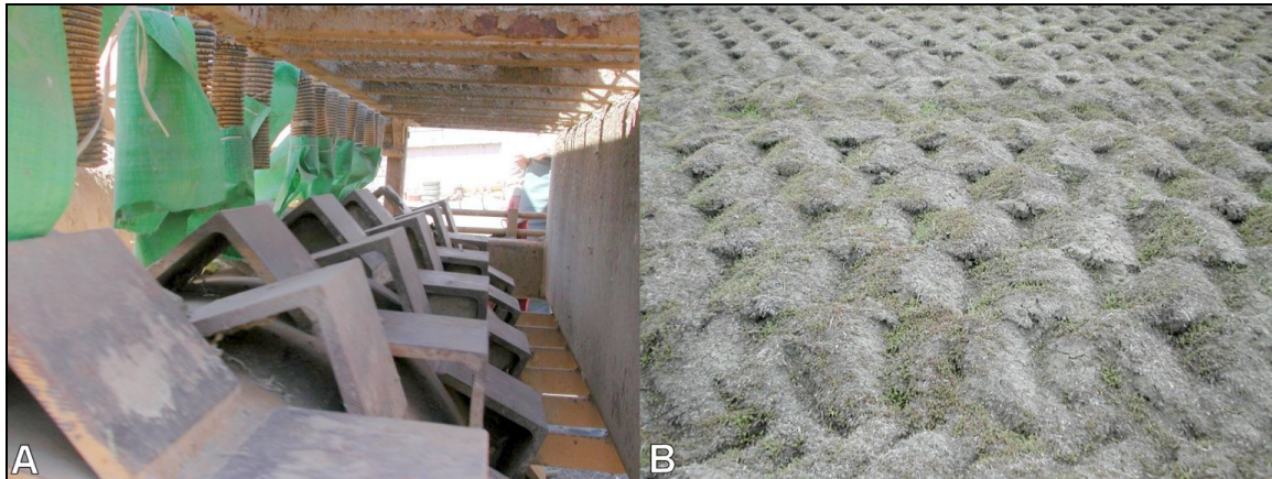
Figure 13. A. Close-up of the teeth on the LRDP imprinter. B. A series of imprints in the clay soil at the Tranquillity site.
